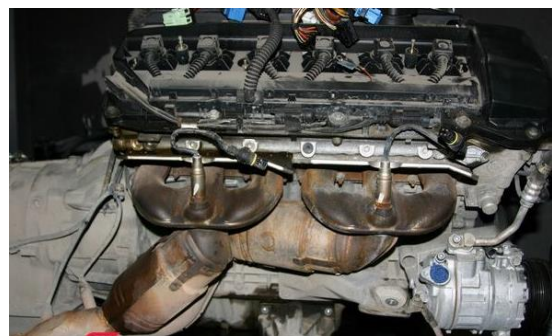
Fig. 2. Factory manifolds mounted on the engine
