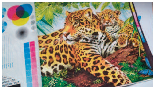
FIG. 5. TEST OBJECTS PRINTED ON A NAPKIN TO DETERMINE DENSITOMETRIC INDICATORS
