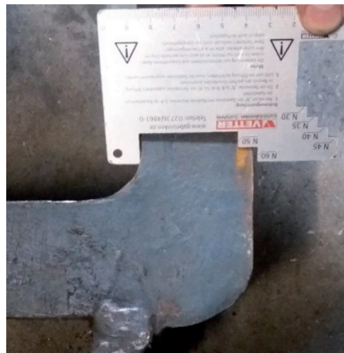
Fig. 6. Inspection of fork tip abrasion using a Vetter straight edge
