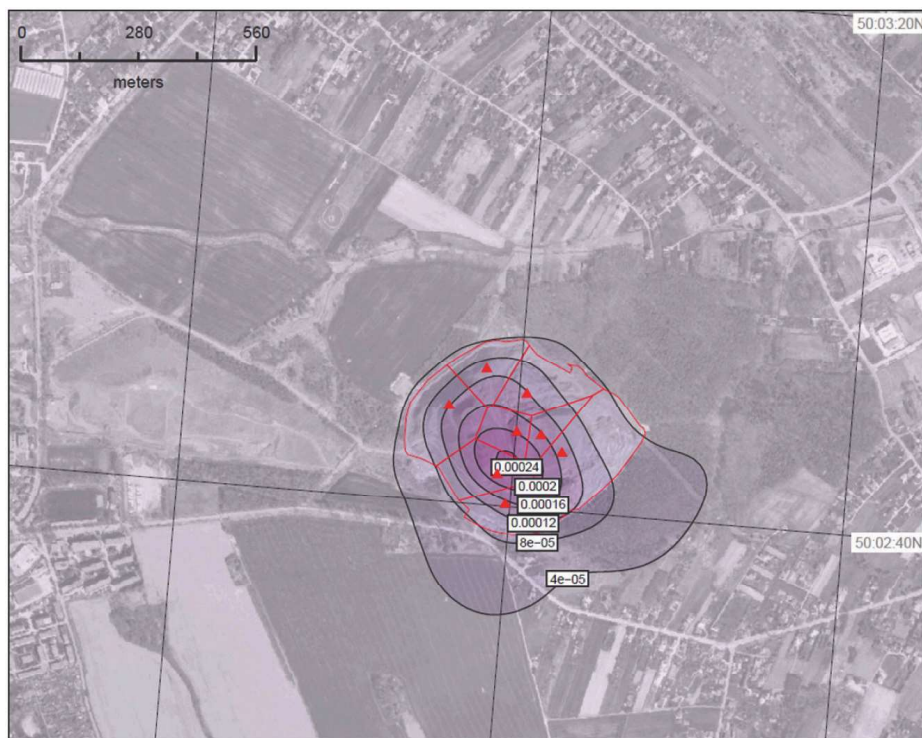
Fig. 8. Pszów location. Total immission contribution to average annual concentrations of B[a]P ( \text{ng}/\text{m}^3 )
