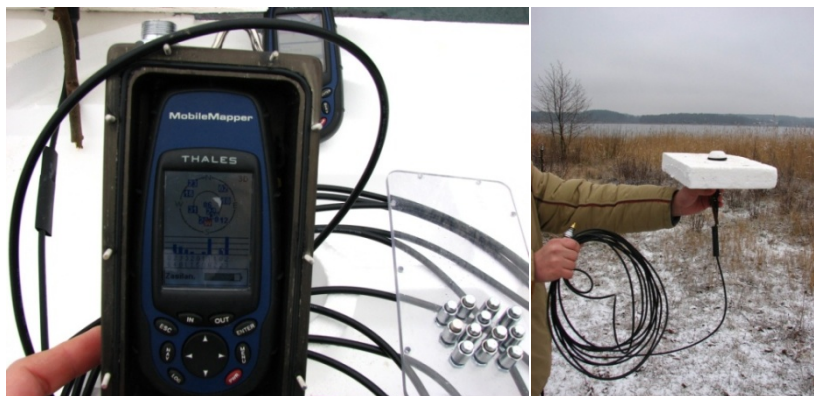
Fig. 3. GPS set: Thales Mobile Mapper in the housing for underwater works. GPS antenna.
