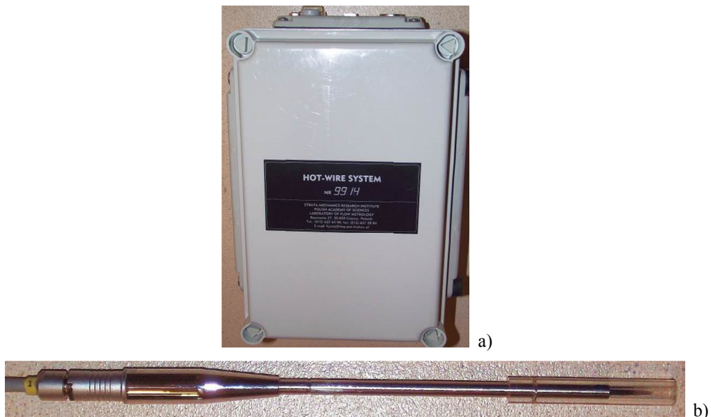
Fig. 3. Multi-channel thermoanemometric system a) with a thermoanemometric probe b)
