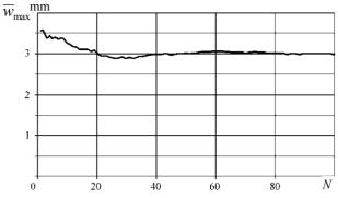
Fig. 3. Alteration of average value of accumulated plate deflection at N = 10 for exponential law of distribution with  $\lambda = 0.07 \text{ N}^{-1}$
