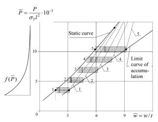
Fig. 2. Modeling the process of accumulation of residual deflection at repeated loading
