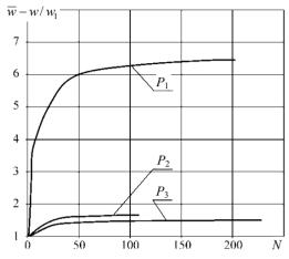
Fig. 1. Accumulation of deflections of loading in variant I
