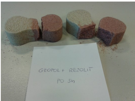
Fig. 5b. Fracture of tensile test specimens of the system: Geopol + Rezolit (after 3h)
