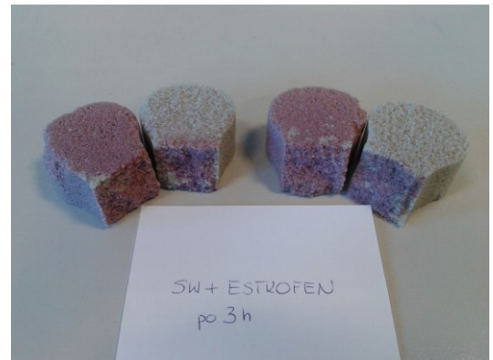
Fig. 5e. Fracture of tensile test specimens of the system: water-glass + Estrofen, after 3h
