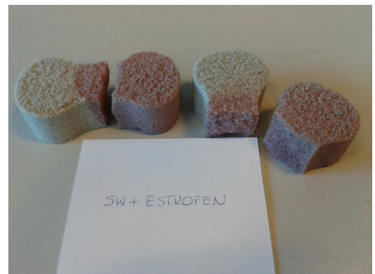
Fig. 5f. Fracture of tensile test specimens of the system: water-glass + Estrofen, after 24h (Contrary to the system Geopol+Rezolit after 3h the fracture occurs at the boundary of two sands, while after 24h in the sand with the Estrofen resin, since the binding of two sands strengthened).
