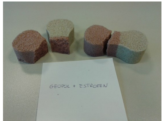
Fig. 5d. Fracture of tensile test specimens – after 24h – for the system: Geopol + Estrofen (The fracture of the tensile test specimen of the system: Geopol+Estrofen after 24h - occurs in the sand with the Estrofen resin)
