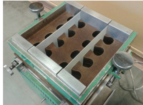
Fig. 2. The way of mounting the partition separating two sands in the LUZ apparatus
