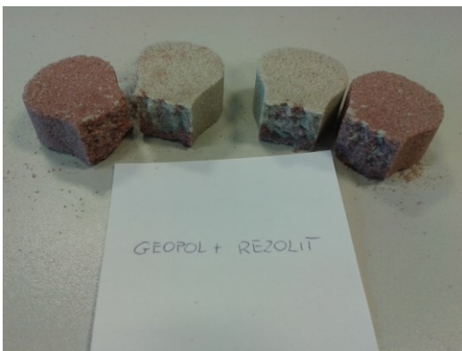
Fig. 5c. Fracture of tensile test specimens - after 24h – of the system: Geopol + Rezolit (The fracture of the tensile test specimen of the system: Geopol+Rezolit after 3h - occurs in the sand with the Rezolit resin, while after 24h - at the boundary of two sands)
