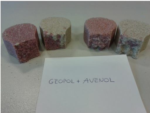
Fig. 5a. Fracture of tensile test specimens - after 24 h - of the system: Geopol + Avenol (Tensile failure occurred at the boundary of two sands)
