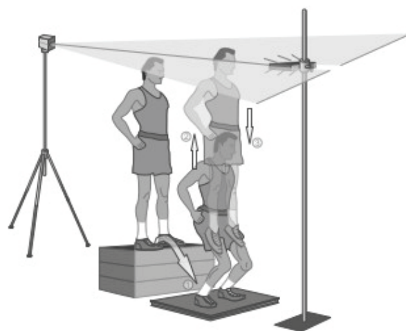
Fig. 1. Display of experimental set up and two methods for controlling the volitional effort. Using an infrared beam from the device that was located behind the subject, the experimenter controlled if the control point that was marked on the subject reached the target jump height. Based on the light signal system which was located in a box in front of him the subject had feedback information whether he jumped to the target jump height
