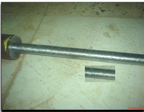
Fig. 9. Poor surface finish
