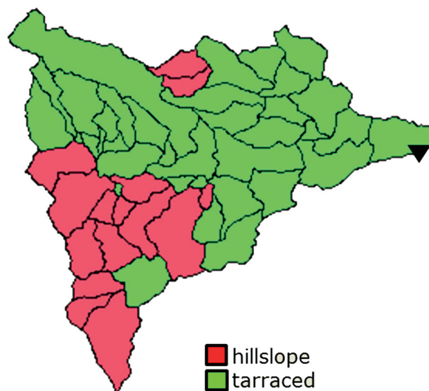
Fig. 7. Delineation of the Bystrzyca Dusznicka into DPR subareas according to HAND procedure
