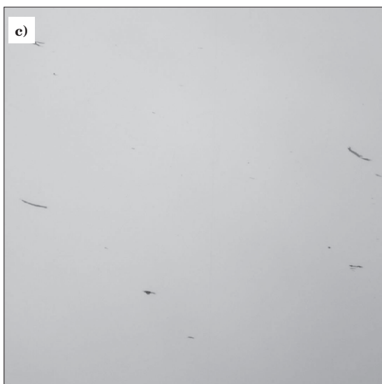
Fig. 7. Non-metallic inclusions in the material without ESR after cold deformation. Tempering temperature of 660°C. Strain rate: (a) 1 s -1 , (b) 10 s -1 , (c) 50 s -1
