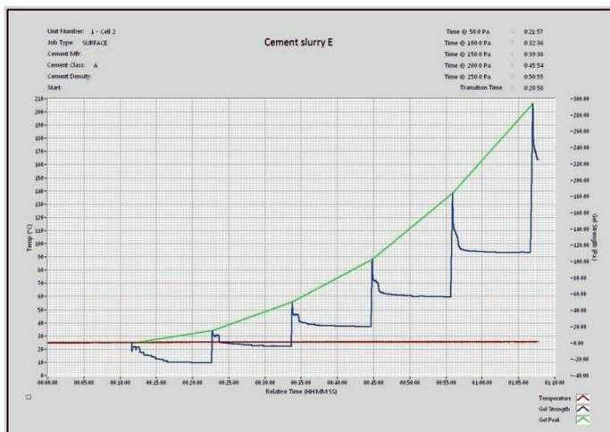
**Fig. 8.** Static gel strength development for cement slurry marked E
