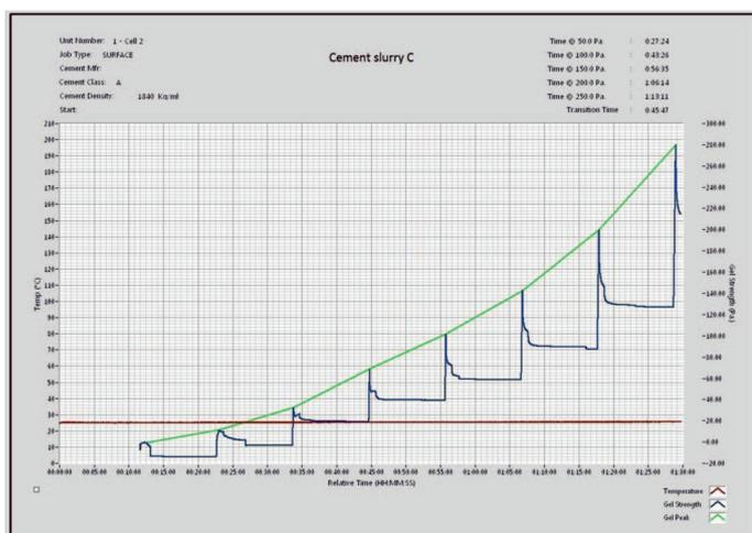
**Fig. 6.** Static gel strength development for cement slurry marked C
