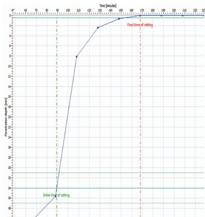
Fig. 15. Thickening time plot for cement slurry F
