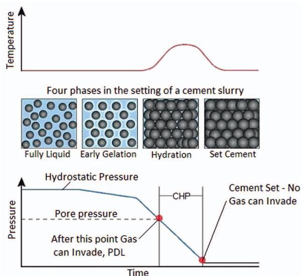
**Fig. 3.** Pressure changes during the setting of the cement slurry in the borehole
