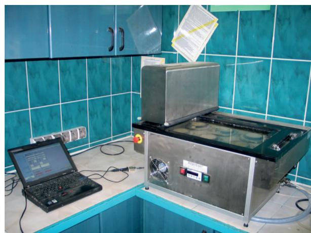
**Photo 1.** Computer-controlled Vicat needle apparatus with 6 measuring points
