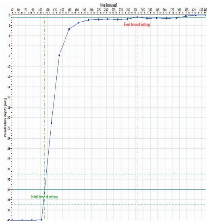
Fig. 14. Thickening time plot for cement slurry E
