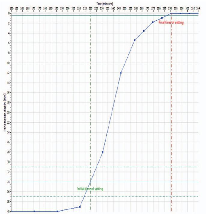
Fig. 13. Thickening time plot for cement slurry D
