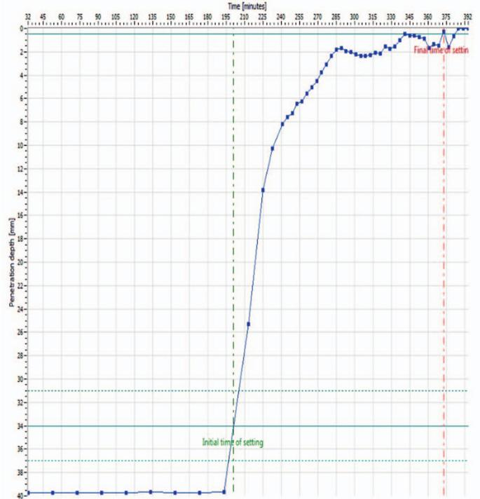
Fig. 11. Thickening time plot for cement slurry B
