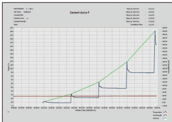
**Fig. 9.** Static gel strength development for cement slurry marked F
