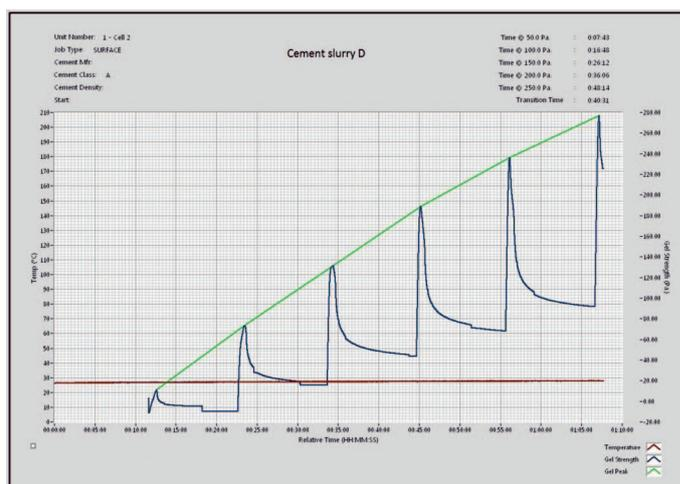
**Fig. 7.** Static gel strength development for cement slurry marked D
