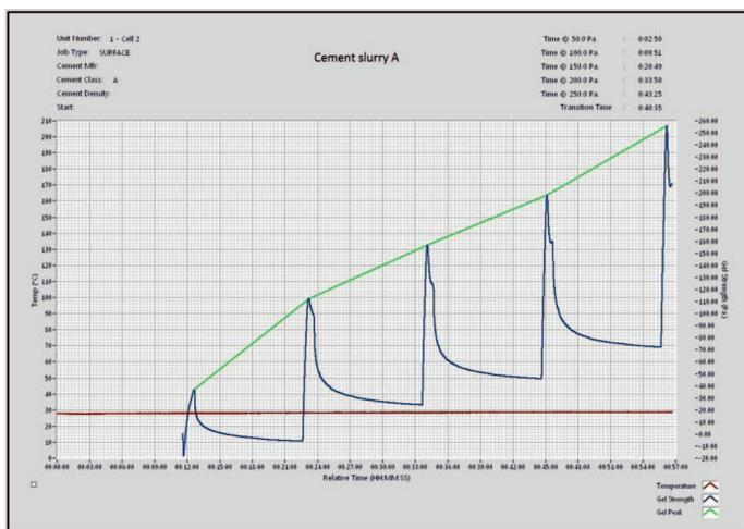
**Fig. 4.** Static gel strength development for cement slurry marked A
