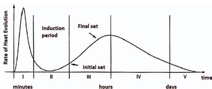
Fig. 1. Hydration curve for  $C_3S$
