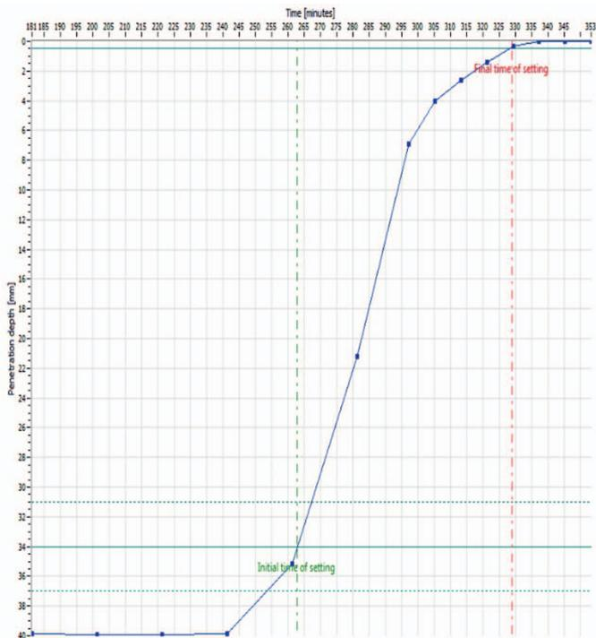
Fig. 12. Thickening time plot for cement slurry C
