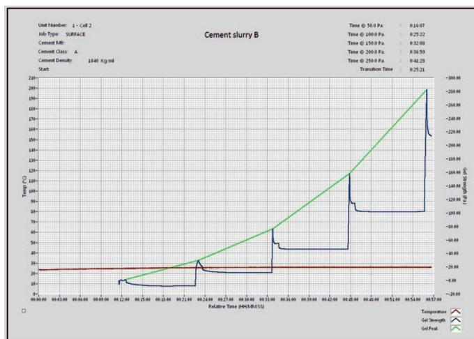
**Fig. 5.** Static gel strength development for cement slurry marked B
