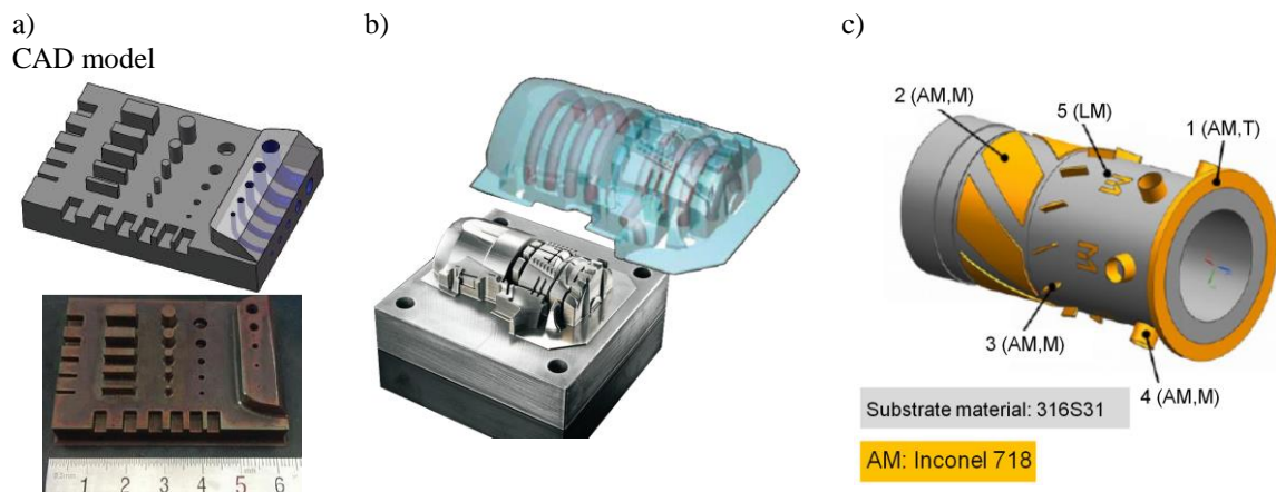
Fig.9. Injection mold with internal cooling channels produced by hybrid A/SM (Additive/Subtractive Manufacturing) process (a), injection mold for the head of electric driver produced by hybrid process including SLM and CNC milling (b) and cylinder shaft for oil industry with locally deposited layers of Inconel 718 alloy (c) [5–6, 8, 16–18]. Symbols: AM/T – additive process plus turning (1), AM/M – additive process plus milling (2, 3, 4), LM – laser marking (5)
