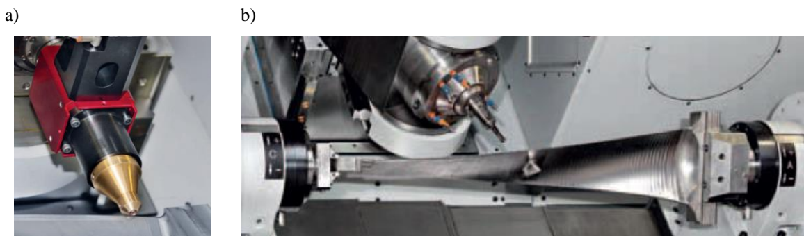
Fig. 17. Remanufacturing of turbine blade: laser deposition of the worn blade edge (a) and subsequent milling of turbine blade after cladding (b) [23]
