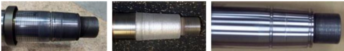
c) material deposition on the undersized forging (atomizer wheel) made of Ti6-4 titanium alloy
