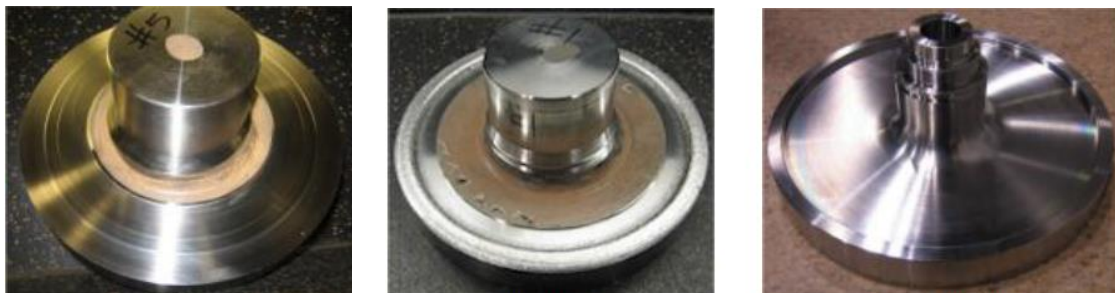
Fig. 20. Examples of repairs of different parts using LDT technique (Laser Deposition Technology) [21], 1 – worn part, 2 – part after cladding, 3 – part after machining of deposited layer
