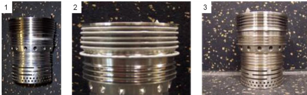
b) regeneration of the atomizer shaft made of 4340 steel, clad material- stainless steel 420 LC
