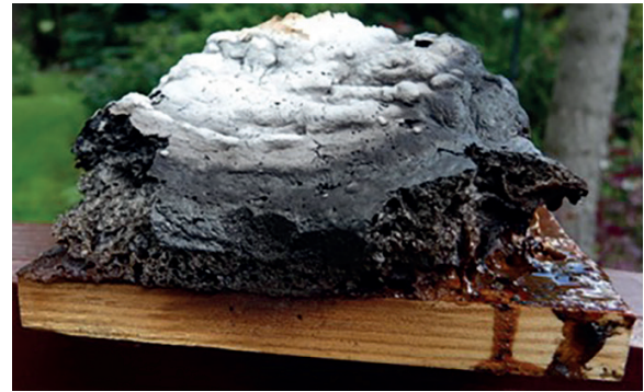
Fig. 6. Ceramic surface with intumescent coating
