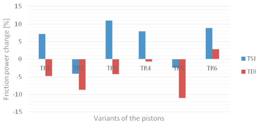
Fig. 7. The percentage difference of friction power for six variants of the piston bearing surface for the SI and CI engines
