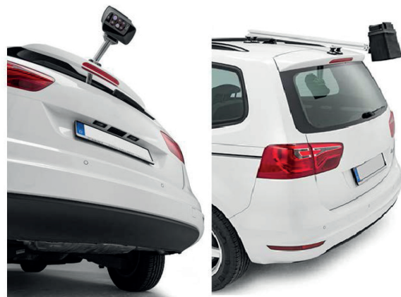
Fig. 1. An exemplary mounting of the mobile sensor [10]
