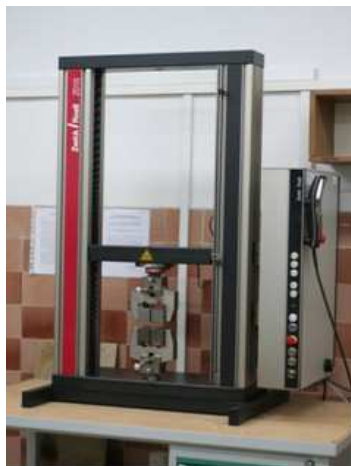
Fig.1. View of: a) an example moulding (the ellipses mark the elements from which samples for the strength tests were taken), b) the Zwick/Roell Z010 universal testing machine
