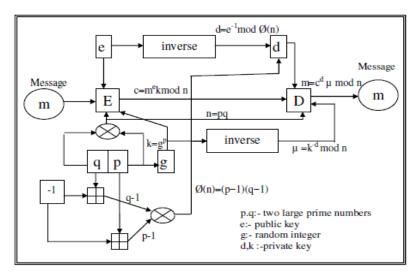
Fig. 3. Process of hybrid public key algorithm
