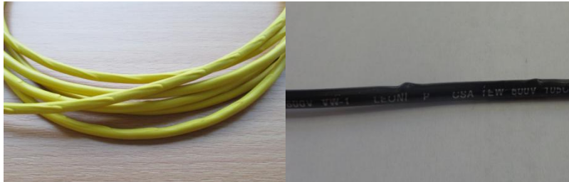
Fig. 7. Cable thickening as a quality defect.
