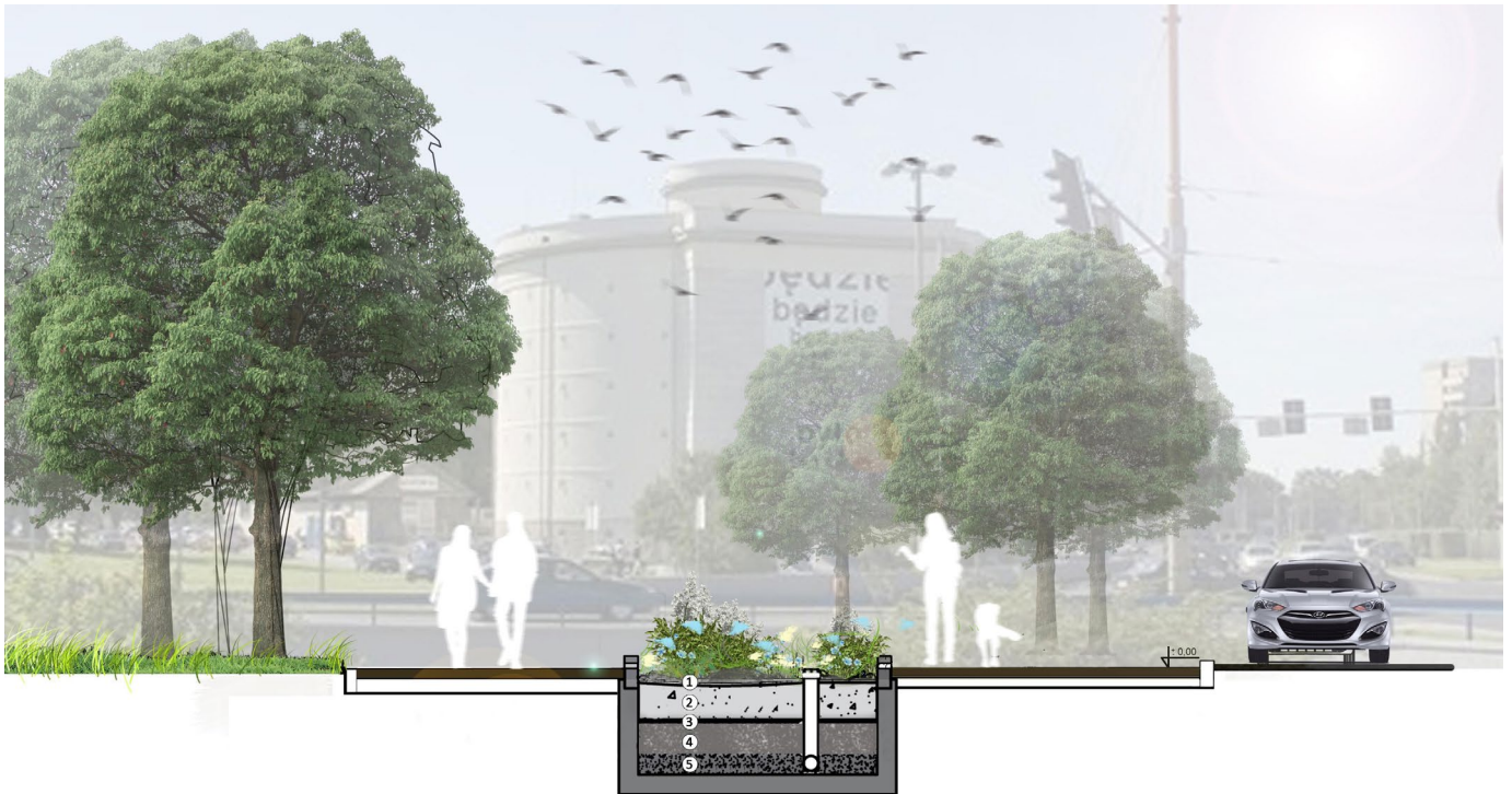
Fig. 8. The rain gardens at the Strzegomski Square and along the string of Legnickiej, Lotniczej i Kosmonautów Streets as an example of environmental solutions in the field of rainwater management (source: the design team's files). Layers of the rain garden: 1. granite grit 8–16 mm – 5 cm; 2. mixture of sand (35 %), ground (35 %), compost (30%) – 50 cm; 3. geotextile 200 g/m 2 ; 4. gravel 16–32 mm – 35 cm.
