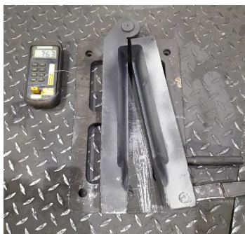
Fig. 3. The shape of the steel mold for collecting test samples
