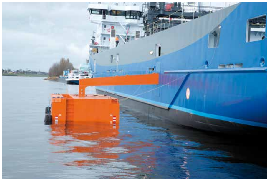
Fig. 5. The Atlantic Dawn with external anti-heeling device [18]
