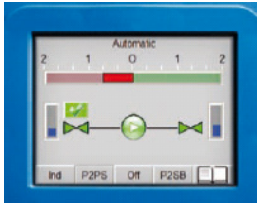
Fig. 1. Visualization of heel (in degree – heel about 1/3 degree on portside)
