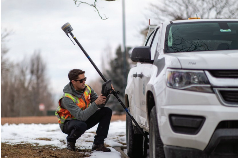
Fig. 5. Measurement using IMU technology
