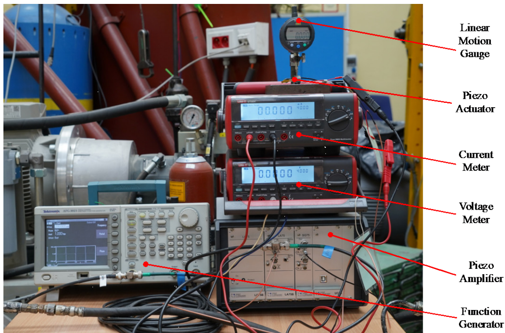
Fig. 2. Piezo-actuator test configuration, source: ILOT
