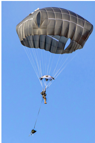
Fig. 8. US troop parachute T-11 with a round slider device [5]
