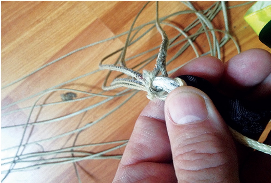
Fig. 2. Severe wear on Vectran Lines [3]
