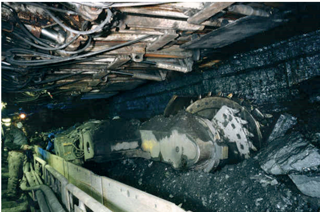
Fig. 3. View of the longwall system during the work
