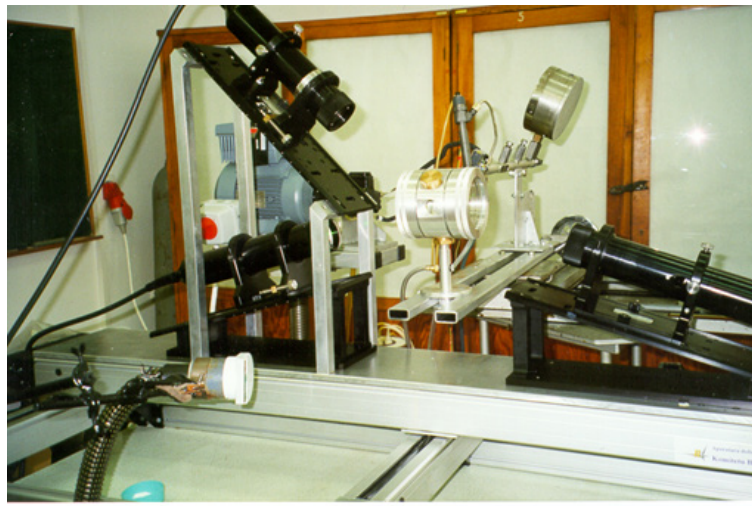
Fig. 2. View of measurement space with injector tested, LDV, PDPA Transducers
