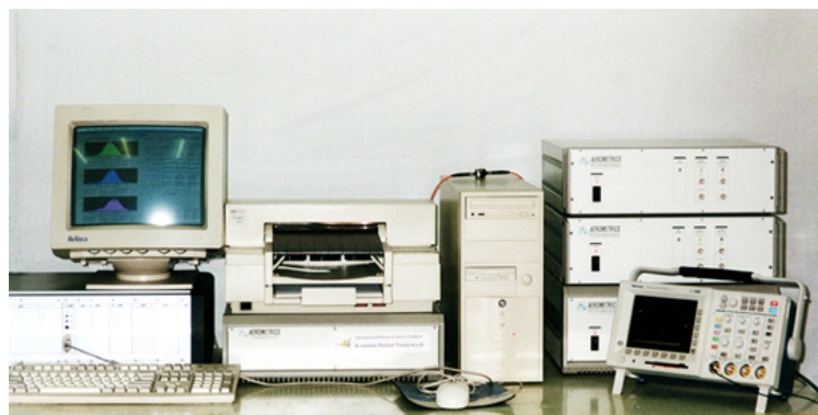
Fig. 3. 3-LDV Analysers, PDPA Analyser, Traverse Programmer, Computer with Printer, Oscilloscope
