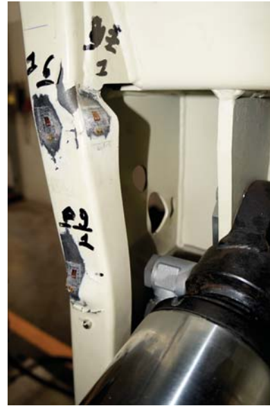
Fig. 15. Deformation of the strain gauge 7 location due to local buckling; note the bulge developing straight at the center of the strain gauge
