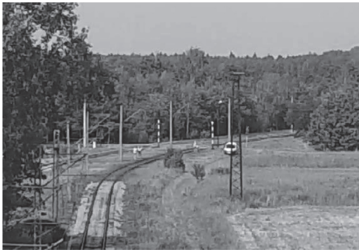
Fig. 7. A frame from the recording of entry signals from a distance of 250 m [own study]
