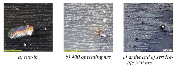
Fig. 10. Spectro T 2 FM ferrograph images showing metal particles in engine oil over the lifetime of an internal combustion engine
