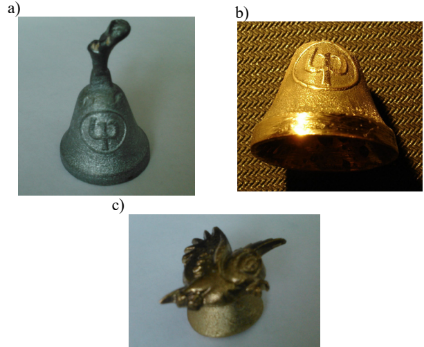
Fig. 7. Castings after knocking out and cleaning: a) ZnAl5, b) CuSn10Pb10, c) CuZn37
