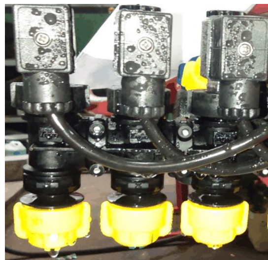
Fig. 2. Head equipped with three solenoid valve-controlled nozzles
