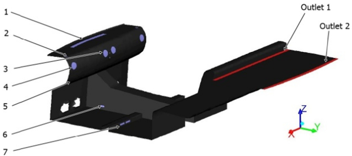
Fig. 4 Position of nozzles inlet and outlets
