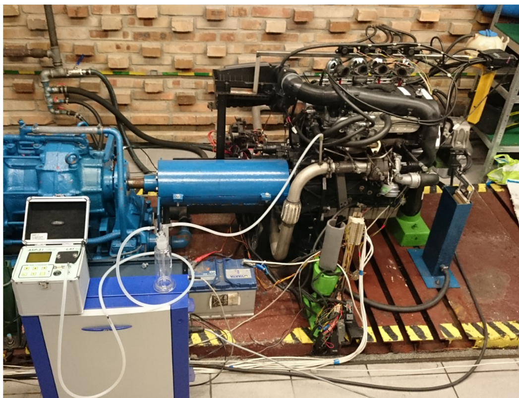
Fig. 1 Measurement system of exhaust compound concentration from Diesel Engine
