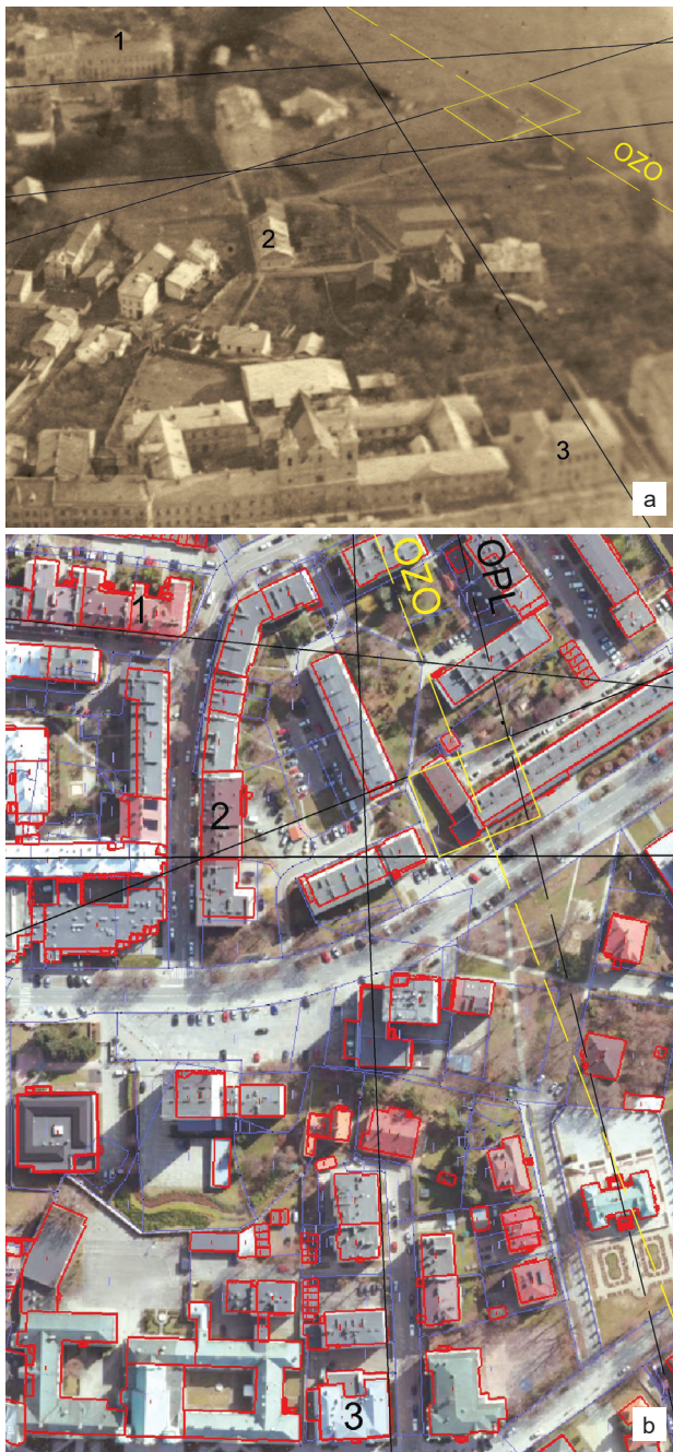
Fig. 8. Reconstruction of the location of the ponds in the garden of the summer palace using an auxiliary planimetric structure: a) aerial photo from 1915 (photo courtesy of J. Rudnicki), b) contemporary map (1, 2, 3 – buildings used in the construction, OZO – axis of the garden layout, OPL – axis of the summer palace) (elaborated by M. Piekarski)
