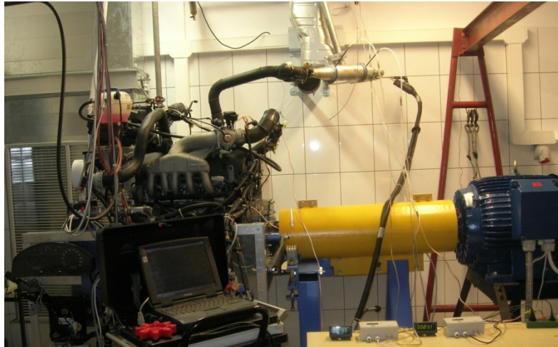
Fig. 4. A view of the TDI engine on test stand during tests on carbon monoxide conversion ratio [13]
