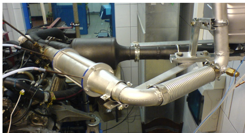
Fig. 5. A view of the exhaust system with a standard oxidizing converter (black housing) and experimental converter (silver housing) connected parallel [13]
