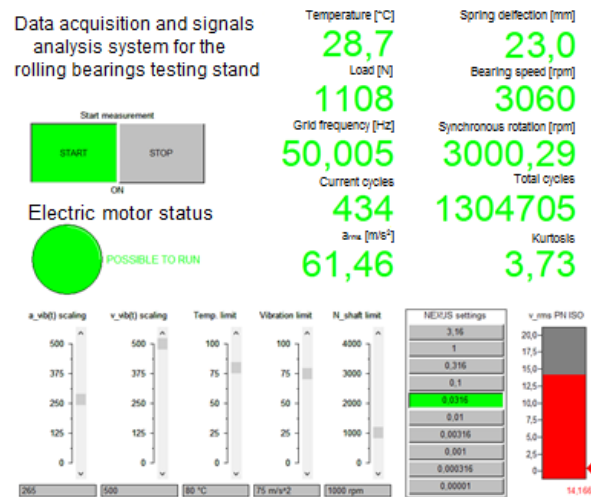
Figure 4. Measurement and control panel of data acquisition and analysis application for the rolling bearings testing stand
