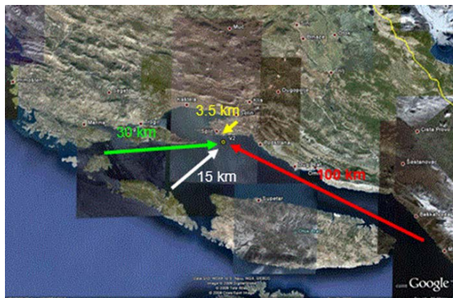
Figure 1. Length of fetch for dominant winds at the station V2 near port of Split.
