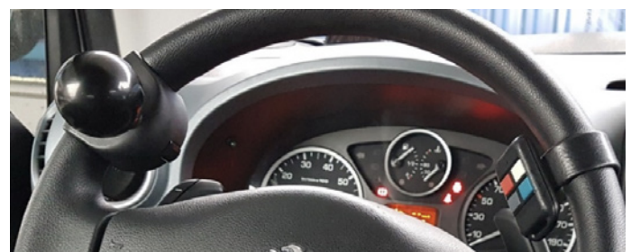
Fig. 4. Knob-shaped handle without remote control function and remote control mounted separately
