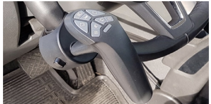
Fig. 3. A handle in the form of a knob with a remote control function
