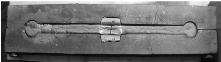
Fig. 23. Metal mould for researching hot tears
