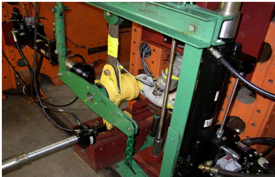
Fig. 4. The main landing gear on a stand during fatigue testing (front-side view). The test is performed in the structural tests laboratory of Polskie Zakłady Lotnicze Sp. z o.o.. The test program [3] was adapted from that prepared by the Institute of Aviation in Warsaw for the previous main landing gear
