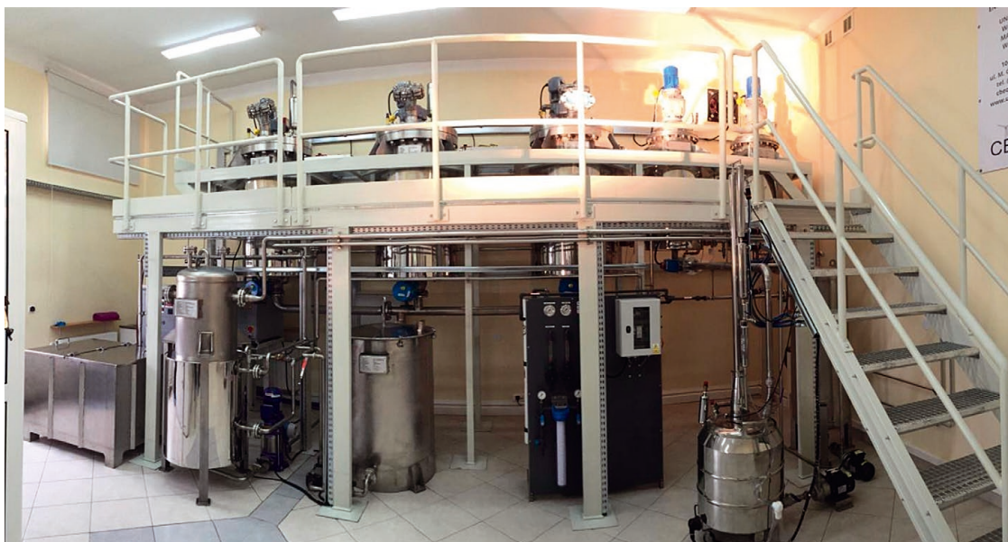
Photo 5. Bio-refinery for the production of second generation bioethanol from lignocellulosic mass [6] (photo by the author)
