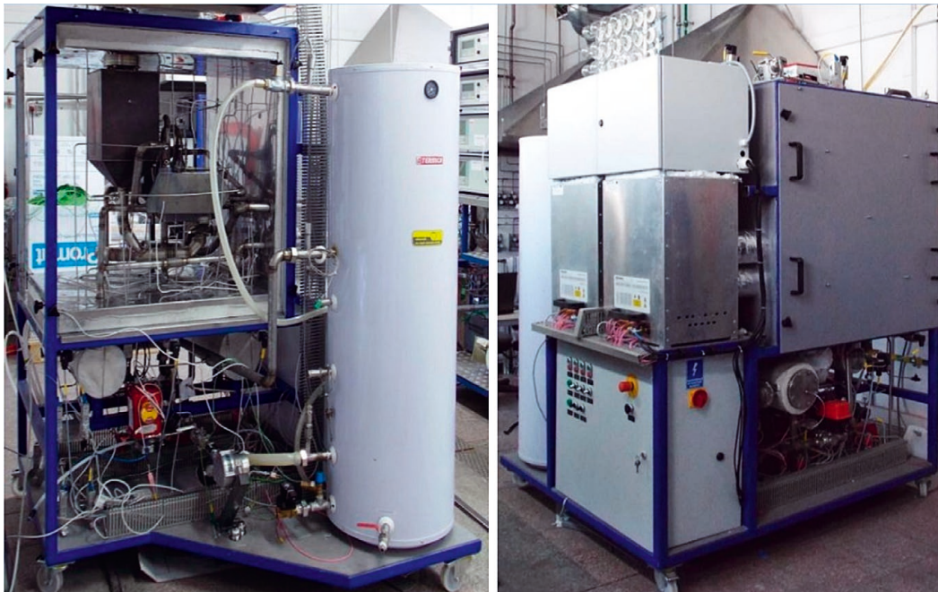
Photo 3. Cogeneration micro-plant with SOFC fuel cells of electrical capacity 2 kW together with a 200 l hot water tank (photo by the author)
