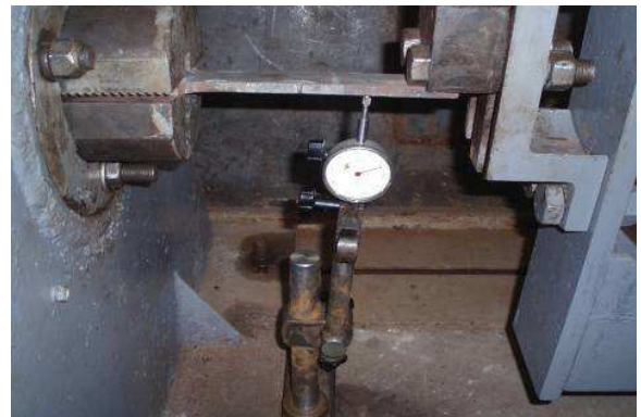
Fig. 4. Sample deflection measurement
