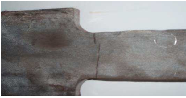
Fig. 5 Moment of crack appear in the experimental sample from metal (1)
