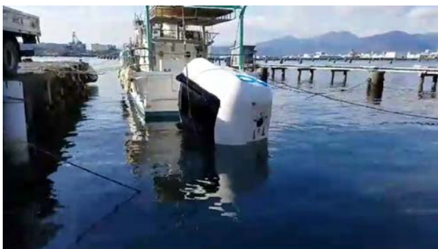
Figure 20. Upside down test in the pier
