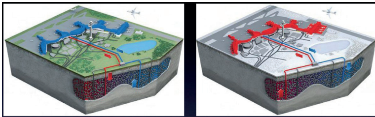
Fig. 9. Example of Aquifer Thermal Energy Storage on the aquifer in Arlanda Airport in Stockholm
