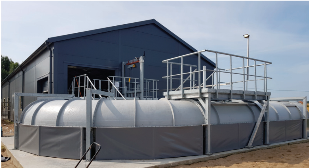
Fig. 3. Photography of the water tunnel
