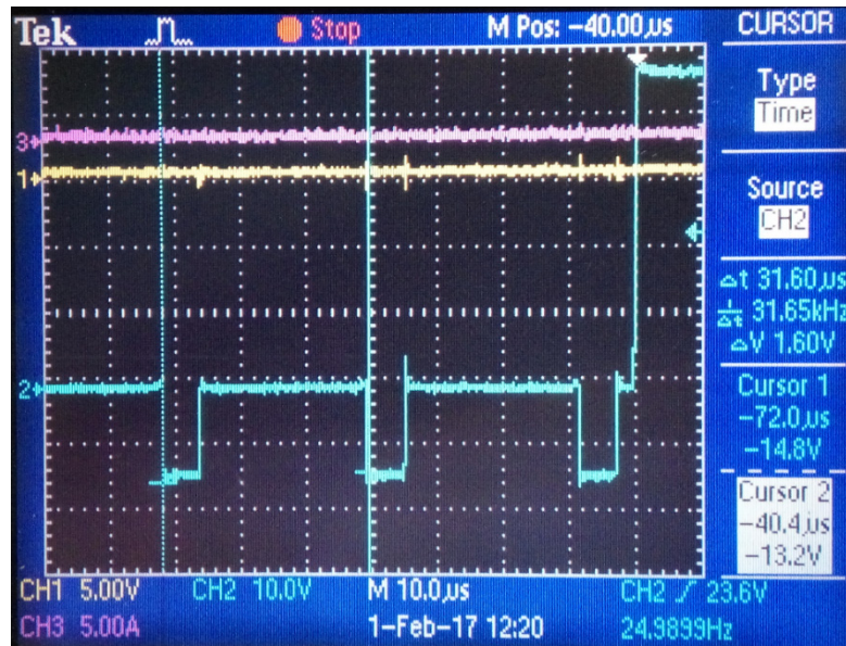
Fig. 9. Control voltage of the Fiat MultiAir system
