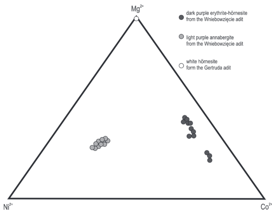
Fig. 8. Ternary plot of the chemical composition of Mg-Co-Ni arsenates from the Gertruda and Wniebowzięcie adits (in atoms per formula units)
