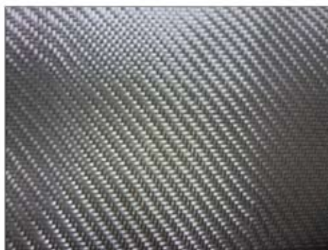
Rys. 2. Tkanina Aeroglass 280 g/m 2 Fig. 2. Glass fabric Aeroglass 280 g/m 2
