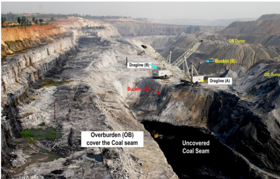
Fig. 5. Draglines in operation sitting at the top of the blasted overburden bench
